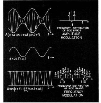
Fig. 2—Diagram of modulated waves and their sideband components for amplitude modulation (top) and frequency modulation.
