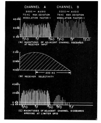
Fig. 6—Amplitude-frequency spectrum of frequency-modulated signals in two adjacent channels, for interfering signal in adjacent channel 6 db greater than desired signal
