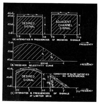
Fig. 5—Graphical study of adjacent channel sideband interference, for adjacent channel 6 db above desired channel signal.
